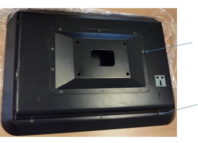
Remove these screws and remove this fitted panel, Mount it on the pillar [with its cross bar for the Side tables), later you can attach this housing after connecting all cables.
