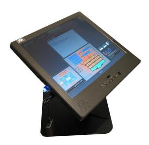
In Table top format, the ILS 1 5RT is the most economical package to present productively and professionally with sho-Q software. The 19" screen is fully interactive with Resistive touch. The integrated PC has 3GHz Dual Core power. Extensive I/O features include DVD, 4 USB, 2 Firewire, SD card reader, PC audio I/O, VGA out, 1 serial port, LAN, PS2 keyboard/mouse ports on solid lectern oriented stand.
