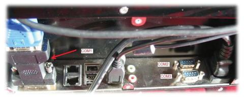
Next to the LAN network connector, the second LAN port can be used to connect to IP protocol driven control systems.
