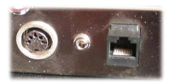
The RPT3 RJ45 has 4 circuits on its 8 connectors that are opened or closed by the relays for any need. Do not apply more than 12 volts per pin pair!
