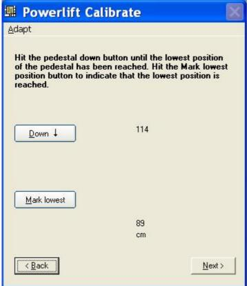
The form shows the approximate lowest and highest position measured in rounded centimeters (in this case 89 cm as lowest and 114 cm as highest). The positions are measured at the front (Presenter side) from ground up to the top of the pedestal.
