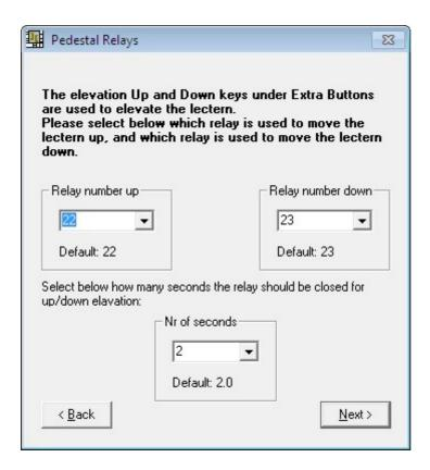
The ILS22 has build-in relays for control functions.
