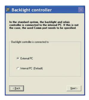
When the ILS22 is delivered in a standard setup, an internal PC is used to control the system and the backlight and relays controller. The internal PC has 4 serial comm ports, of which COM4 is used to communicate with the backlight controller (see above scheme). In situations where an external PC is used, ILStranslator needs to know to which serial port will be used to address the backlight controller inside the ILS22.
