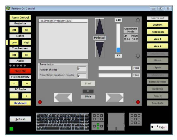
Note that the keyboard backlight is off, indicating the keyboard is disabled. Specifically note that the up and down arrows are now green back lighted, both on the lectern and as here indicated via Remote-Q. The presenter can now press and hold the arrow up key to move the pedestal up, until released again. Same applies for the arrow down key.
