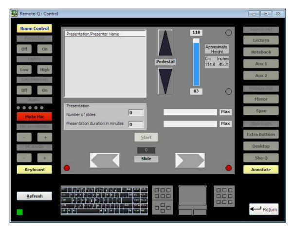
Annotate. Will enable the annotation keys on the ILS22. This will allow the presenter to capture (New Sheet), annotate current captured images, either PowerPoint, Excel, Word, Internet accessed resources or any other, and save it for distribution. The other way around, the Remote-Q operator will see if the annotation keys were enabled on the ILS22 (which is true for all presenter button hits).
