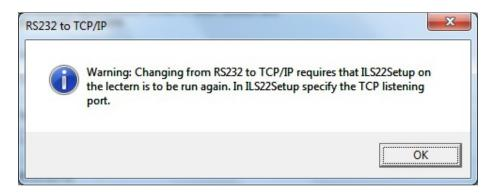
If ILStranslator was setup to allow control access over TCP/IP and you hit the Connect button under the ILStranslator TCP port, Remote-Q will try to verify whether the IP address complies with the standard and whether the TCP port is in the correct range, and than try to make a connection.
