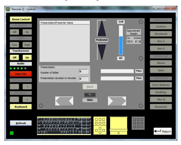
The above image represents the status after hitting the Room Control key once, either by the operator of Remote-Q or the presenter behind the lectern, with the Room Control mode set to carrousel (ILStranslator/Setup/Sequence). Note that the Touchscreen header is now enabled and the Off and On buttons below it are too. Also note that the Audio header function is enabled. In this example we hit it to obtain the ILS22 Audio volume setting, indicated by the
